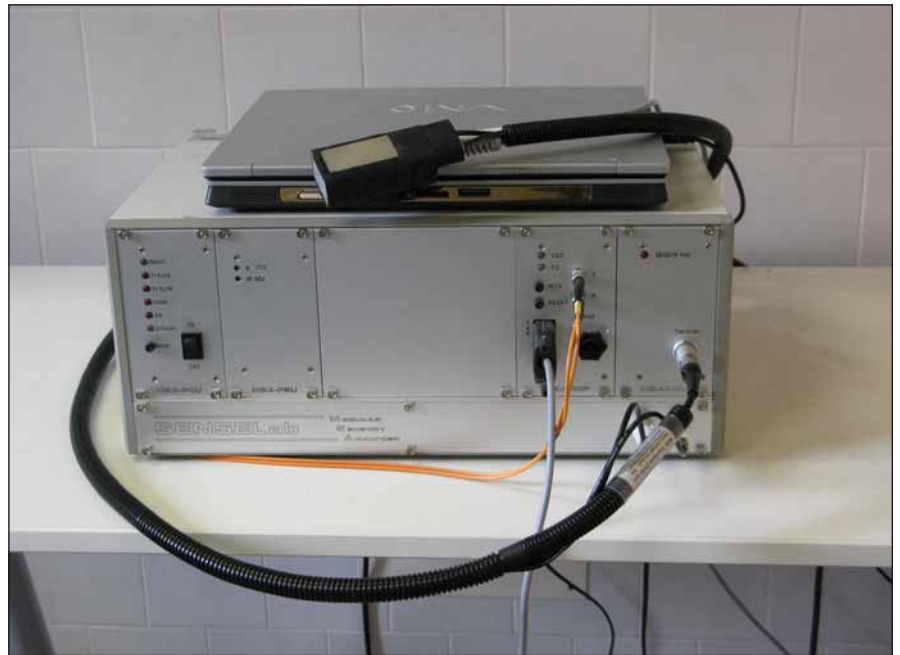
Obr. 1. Teplotní stimulátor SENSELab – TERMOTEST MSA, Somedic, termoda 25 × 50 mm. Fig. 1. Thermal stimulator SENSELab – TERMOTEST MSA, Somedic, Thermode 25 × 50 mm.
